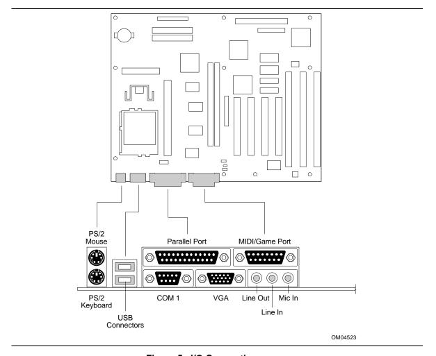
Figure 5. I/O Connections
